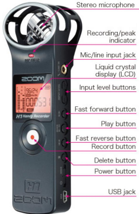
The Zoom H1 is an affordable portable stereo recording device. On the front end, it is equipped with an excellent stereo XY microphone setup capable of recording very high quality sound.
